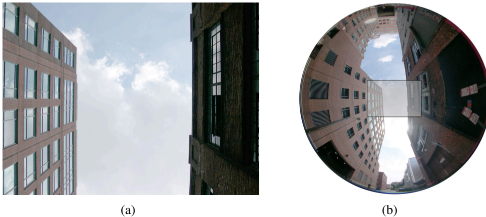
Figure 1.2: Comparison of a perspective image (a) and an omni-directional image (b) taken from the same location. The perspective image contains only a very small skyline compared to a much larger one from the omni-directional image. As a result, the localization using perspective images can be extremely ambiguous. The marked rectangle shows the overlap between the perspective and the fisheye image.
