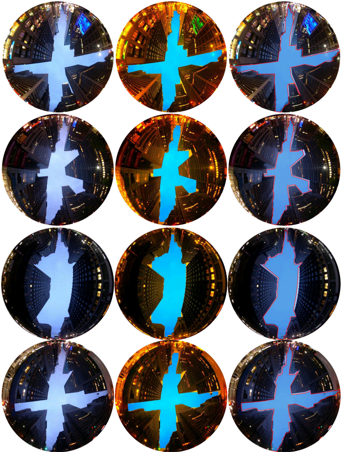
Figure 5.7: Some results of the matching algorithm for the New York data set. The rows show in order the original, the sky detected and the skyline matched images (ordered from left to right).
