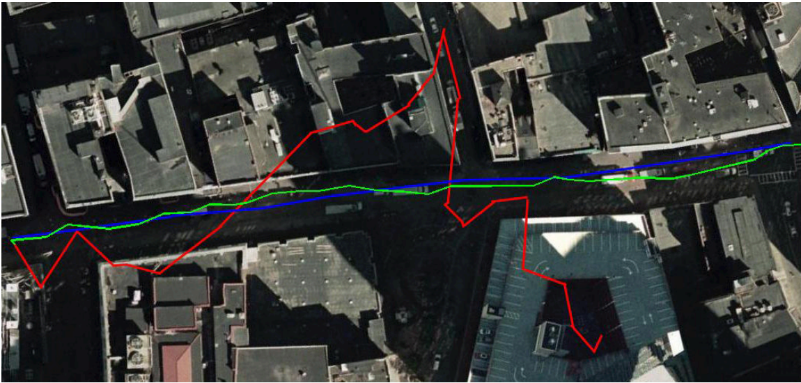
Figure 5.10: We compare the accuracy of commercial GPS units and our fisheye-based system in the Financial District (tall buildings) using 31 sample points. The blue line shows the ground truth (although not completely accurate as it is manually marked on the boundary between the road and sidewalk), and the red and green lines mark the piece-wise linear curves of 31 points obtained from GPS measurements and skyline-based geolocation respectively.
