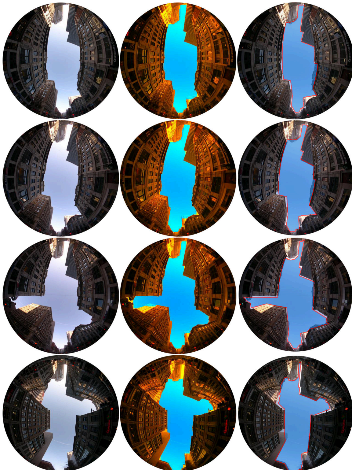
Figure 5.6: Some results of the matching algorithm for the Boston data set. The rows show in order the original, the sky detected and the skyline matched images (ordered from left to right).
