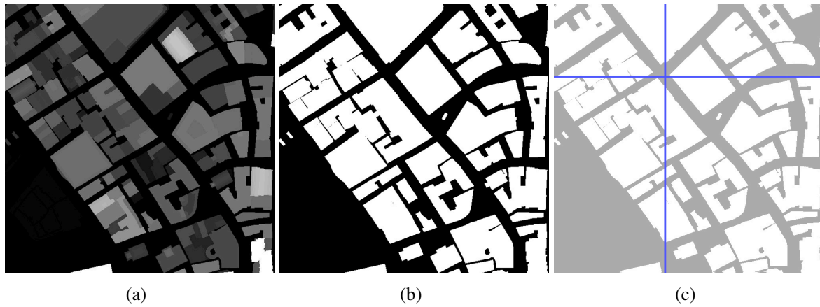
Figure 4.4: The various steps in creating an aerial image displaying buildings and roads from the 3D model of a city (a) Orthographic depth map (b) Detection of buildings using the Z values (c) Localization of the car on the aerial image.
